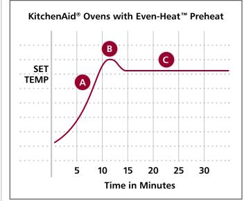
Powerful elements heat the oven above the set temperature to saturate the oven walls and racks with heat, eliminating cold spots before preheating is finished.
